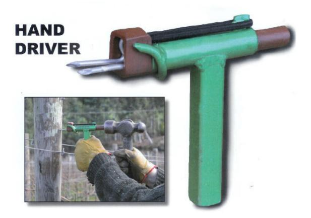
The Tuckaway Hand Driver is useful as either an entry-level or small scale installation tool, as well as being invaluable to users who want a convenient portable alternative to Pneumatic installation for touch-up or post replacement jobs.
