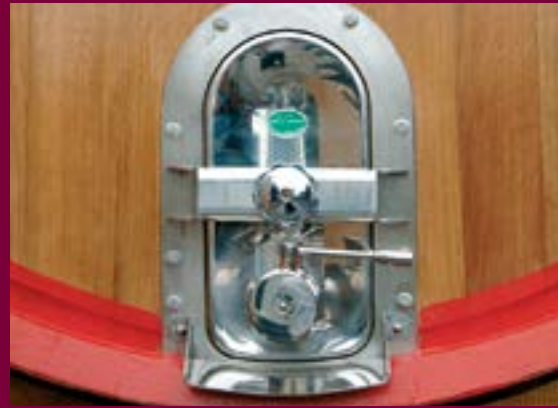
Stainless steel door 18/8 AISI 304 Size 24 x 46 cm, easy to reach, complete with the valve requested. Fitted perfectly into one special central stave at the bottom end of the cask.
