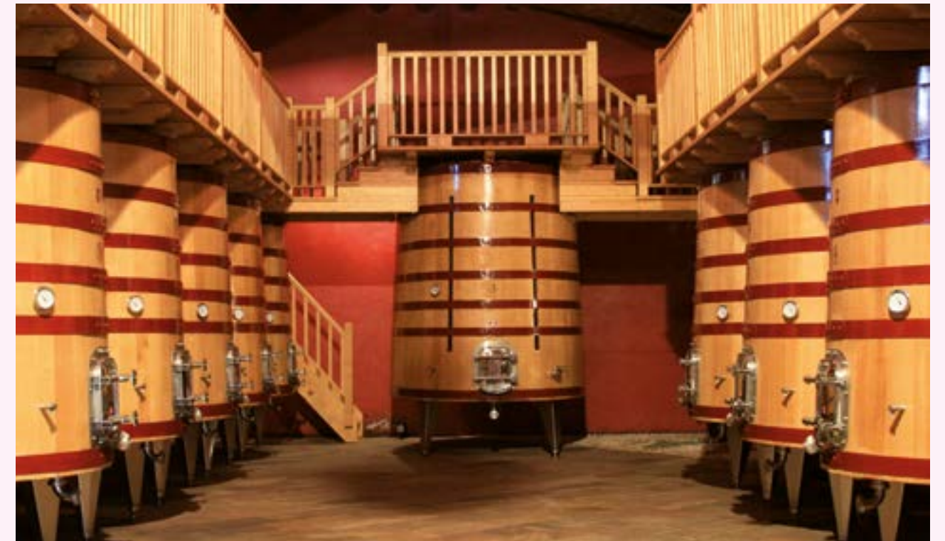
Vat capacity 50 hl and 100 hl with bottom level door.
