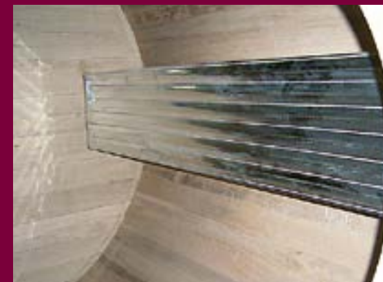
Heating pipes Made of stainless steel 18/10 AISI 316 plates with double welding system and probe shaft. It can be fitted horizontally or vertically depending on the height of the vat. One plate for every 50 hl holding capacity.
