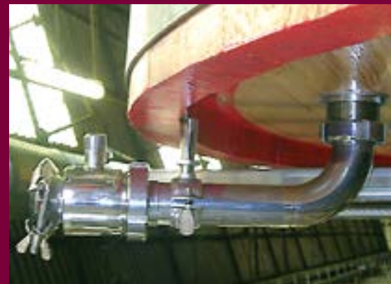
Total drainage pipe in stainless steel 18/8 AISI 304 Complete with final valve as requested, fitted to one central stave at the bottom of the vat.
