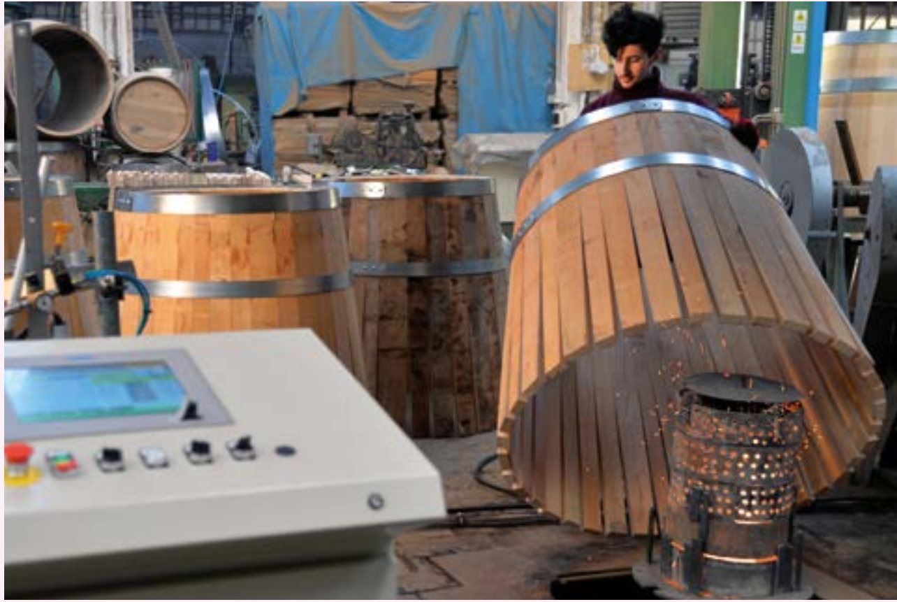
Bending using a direct flame with Digital Toasting System®.
