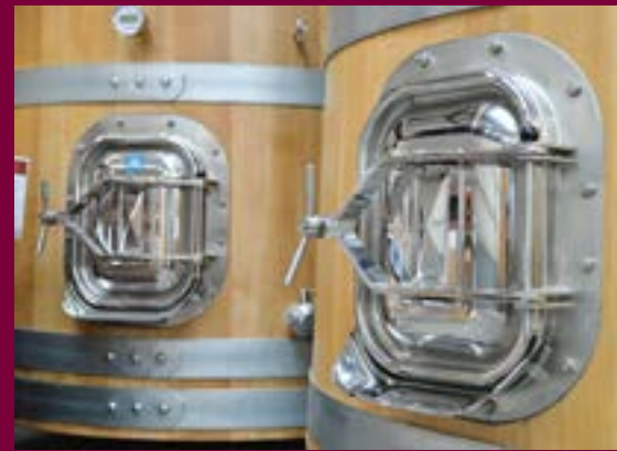
Stainless steel door 18/8 AISI 304 Fitted at 30 cm from the bottom 31 x 42 cm measure, easy to reach, opening outwards.
