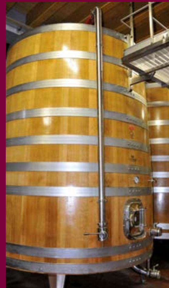
Purping over Pumping over system.
