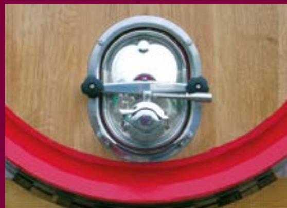
Stainless steel 18/8 304 door (for small casks) Size 19 x 26 cm, inserted at 3 cm from the top of the staves, complete with steel valves.
