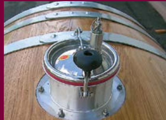
Stainless steel 18/10 AISI 316 bung-hole stopper 16-22 cm diameter, 9 cm high, complete with pressure valve in steel or moplen. Total drainage pipe in stainless steel.
