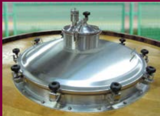
Stainless steel 18/10 AISI 316 convex upper bung-hole cover Dimension in proportion to the diameter of the vat from 40 to 120 cm. Available in 2 versions: central with relative filling-up hole or with 22 cm diameter escape pipe complete with pressure valve.
